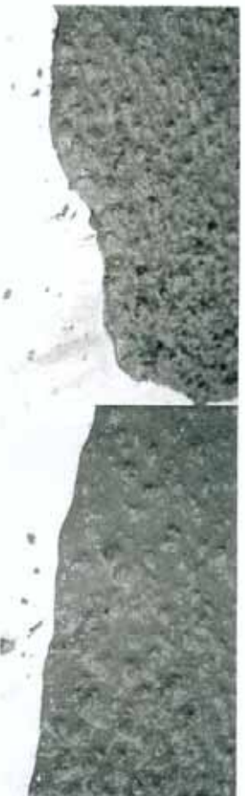
Fig. 5: Appearance of (a) reference concrete and (b) smart dynamic concrete in plant B
